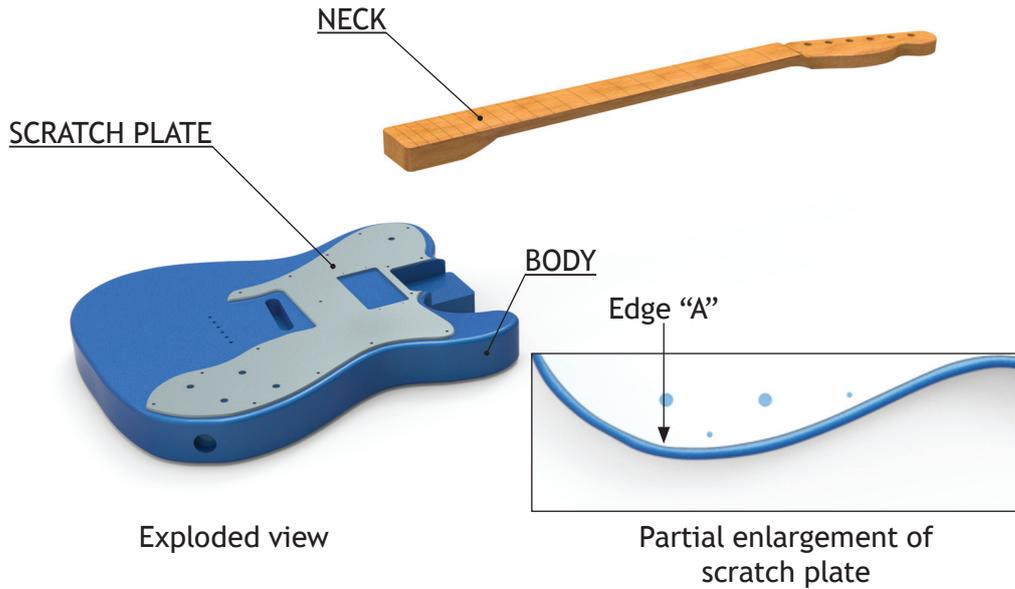
The CAD technician used the process of **top down modelling** to ensure the neck would fit with the body.
