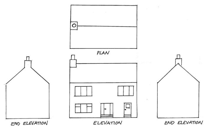
The example above shows four **Orthographic** views of a typical house. Things to note are:
