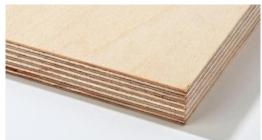
**Plywood**—made by gluing thin layers of wood together. Each layer has the **grain** going at **right angles** to the layer above and below. This makes it very **strong**. Depending on the type of glue used, plywood can be **waterproof** (often called marine ply). Plywood has a good strength to weight ration. As it is glued in layers, it doesn't twist or warp.
