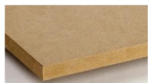
**MDF**—made by mixing a plastic resin with wood fibres or wood flour. It stands for **medium density fibreboard**. The board is very stable and has a good surface that is easy to paint. The dust from mdf, due to the resin, can cause health issues.
