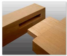
The Mortise and Tenon joint is often used when making tables and chairs. The **tenon** is cut into the rail, and this tenon is then inserted into a square hole named a **mortise**. Traditionally, mortises were cut out using a **mortise chisel**. These were made with heavy blades, so that they could be hit hard with a mallet. Cutting a mortise this way took a lot of effort and was difficult to do.
