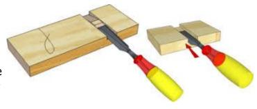
Turn round the timber and repeat from the other side. You should end up with a hump or roof shape in the middle.
