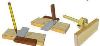
Set your **Marking Gauge** to the depth of the housing joint. This is usually something between one third and one half of the thickness of the first piece of wood.
