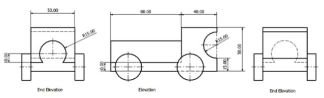
Drawings of a simple toy train are shown above. The train is made out of one single piece (i.e., there are no parts). Make a Modelling Plan to show how to build the toy train. You will probably have a minimum of eight stages.
