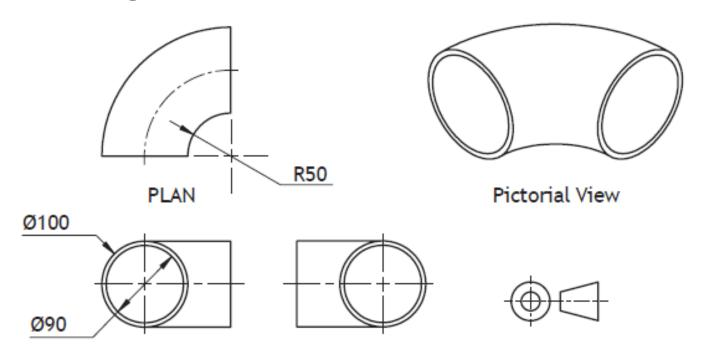
Orthographic drawings and a pictorial view of a type of plastic pipe-corner is shown above.
