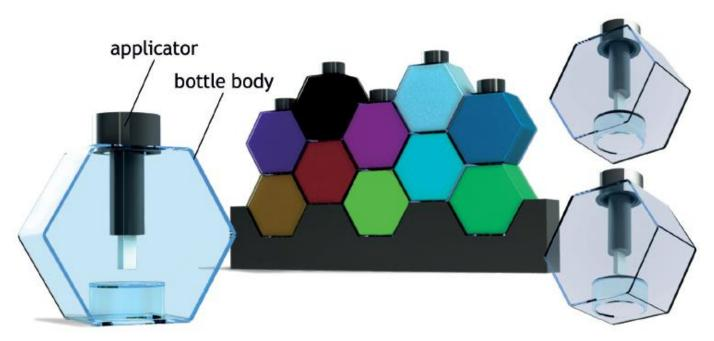
A new line of nail varnishes has been produced by a cosmetics manufacturer. The bottles are stackable for ease of storage and display. 3D CAD illustrations are shown above.
